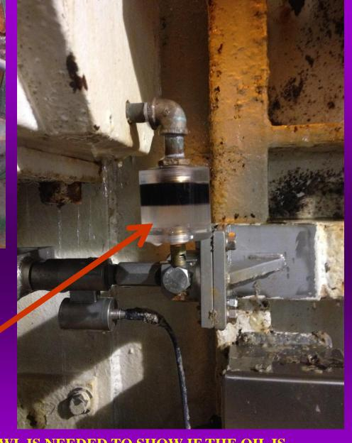
OIL CONDITION SIGHT GLASS OR BS&W BOWL IS NEEDED TO SHOW IF THE OIL IS SATURATED W/WATER, THE OIL HAS FREE WATER, AND THE OIL LEVEL IS POSSIBLY TOO HIGH.
