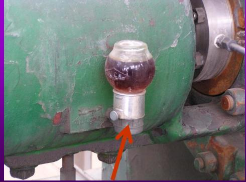
OILERS CAN PROTECT AND CONTAMINATE THE LUBRICATING SYSTEM.
