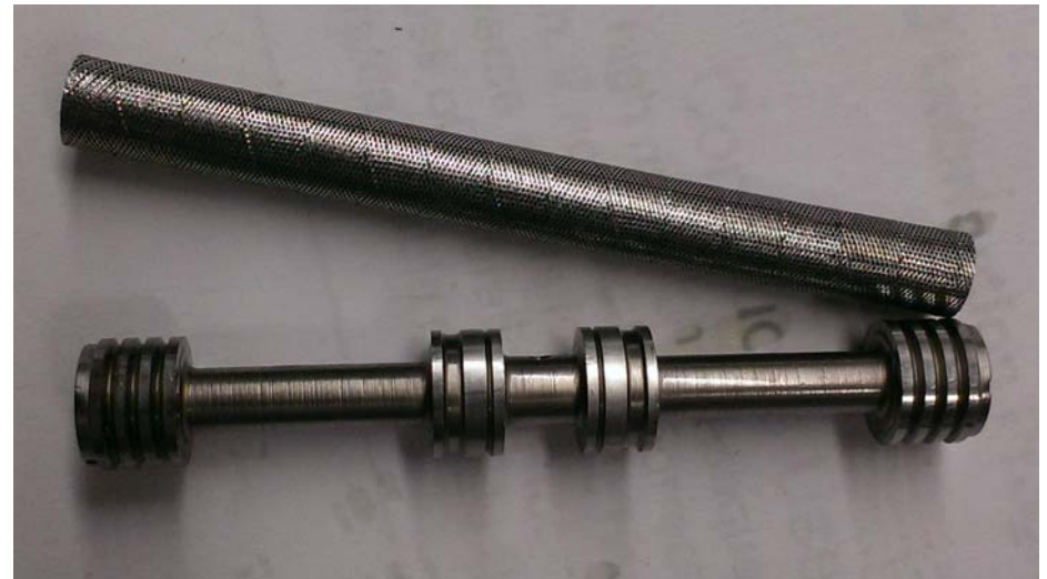
Clean Pencil Filter & Valve Spool
