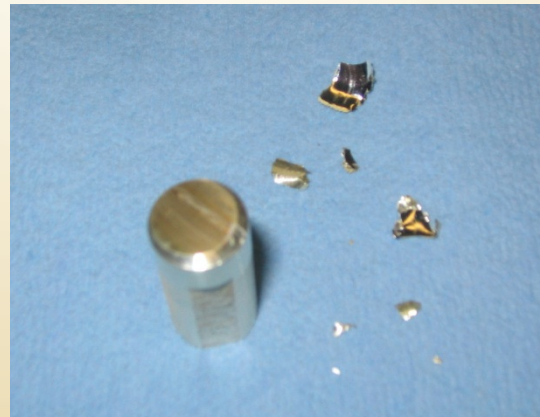
Unexpected Laminar Pin Debris in Cryo Tests
