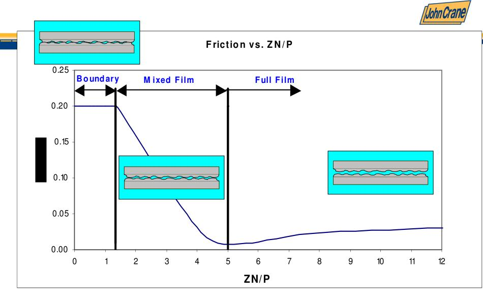
Z = Dynamic Viscosity of Lubricant at Supply Temperature (cp); N = Rotational Speed (rpm); P = Specific Load on the Bearing (psi)
