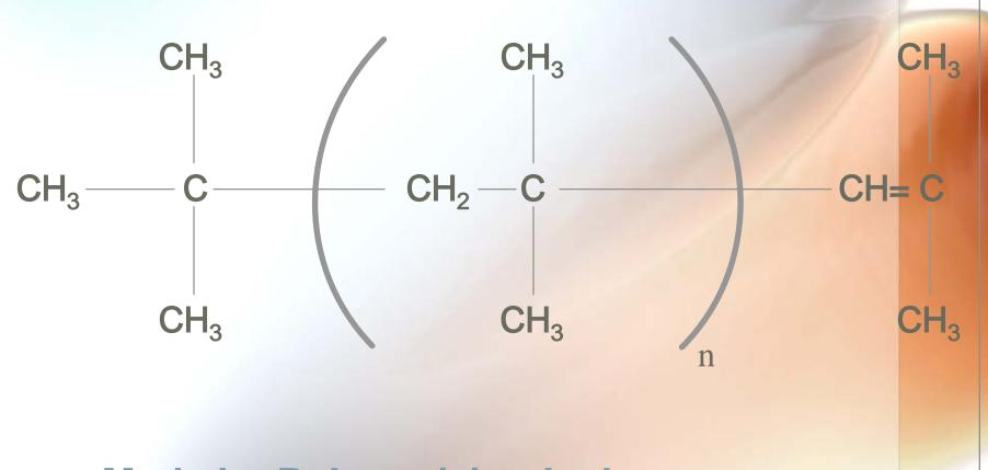
Made by Polymerizing Isobutene
